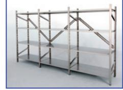
When calculating size, the following must be taken into account: L width of the shelf – D depth of the cross member – H height of the side. The slot joint between a linear cross member and upright improves stability with respect to the weight it carries, while the shelves are independent and can be moved, removed or added without needing to adjust any other element.
